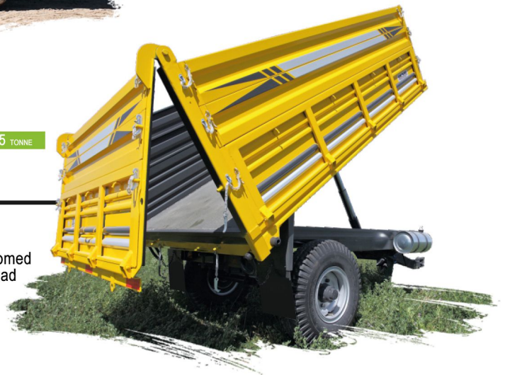
AOT 401H 6 TONNE Single-Axle Monocoque Trailer
